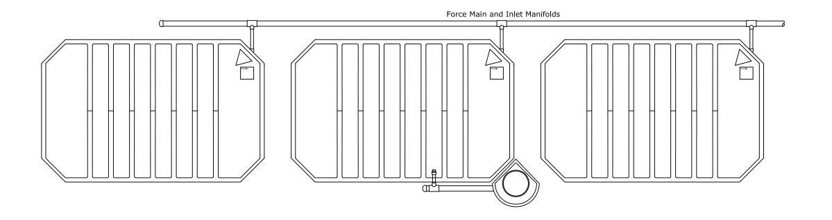
1) BLUE CODED MODULES WITH WEEP HOLES AND ONE GREEN CODED MODULE WITH SAMPLING CHAMBER, DRAIN INTO A STONE PAD FOR FINAL TREATED EFFLUENT DISPOSAL
